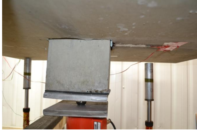
Fig 4 Punching of column in the flat slab after failure.
