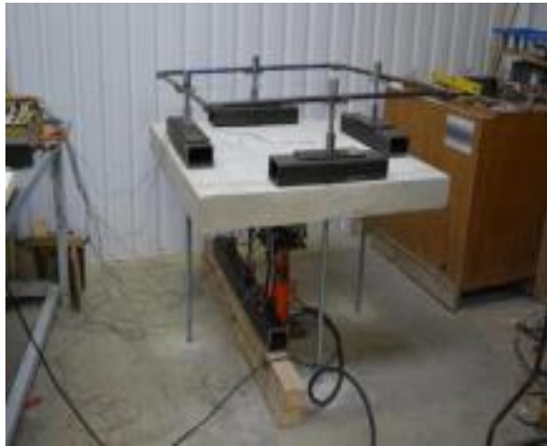
Figure 1: Schematic diagram of testing arrangements of flat slabs
