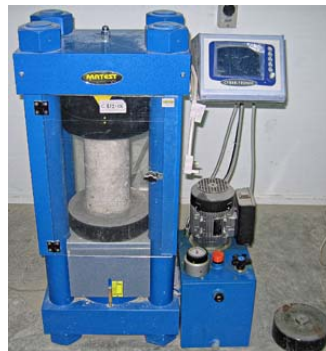
Fig. 1. Testing setup for measuring the compressive strength of concrete
