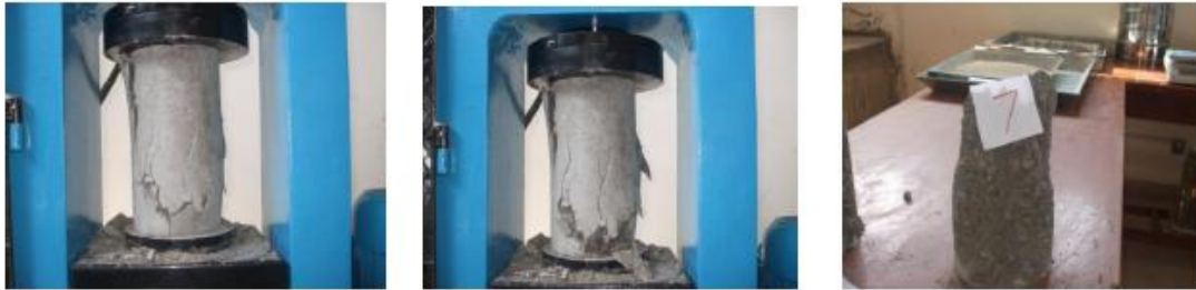
Fig. 5 Details of cracked sections and cracking pattern of natural aggregates concrete
