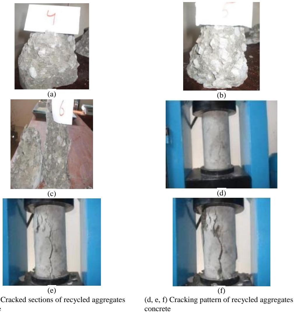
Fig. 4 Details of cracked sections and cracking pattern of recycled aggregates concrete
