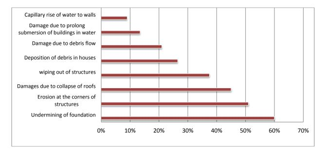
Fig. 3. Major causes of collapse of the mud houses in the flood affected areas.
