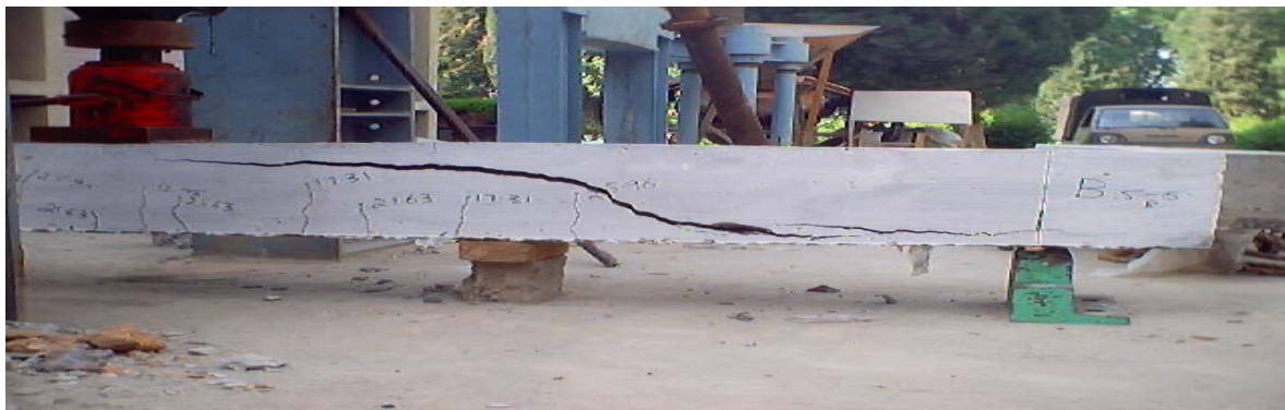
Figure 5. Typical shear failure of beam without web reinforcement. The failure is more brittle and sudden. Brick has been placed under the beam to avoid its splitting in two parts ( \rho = 1.5\% , a/d = 5.5 span = 321 cm).
