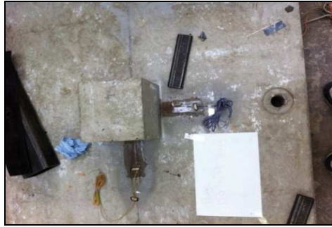
Figure 20 Concrete strain gauges on compression face of slab
