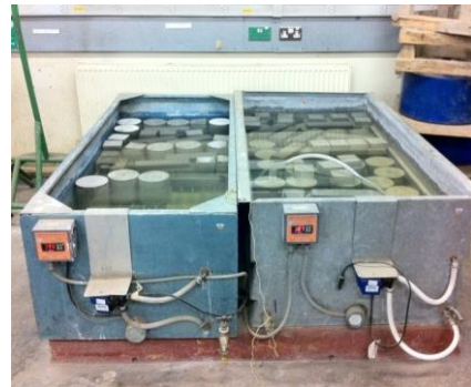
c. water curing environment (C3)
