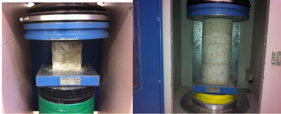
Figure 1 Compressive strength Test using Avery Denison 2500 kN machines
