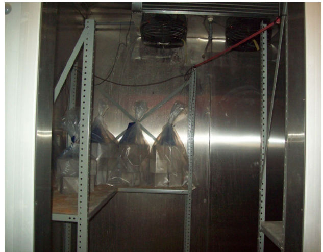
Figure 4. Test cubes under winter curing environment (C2).
