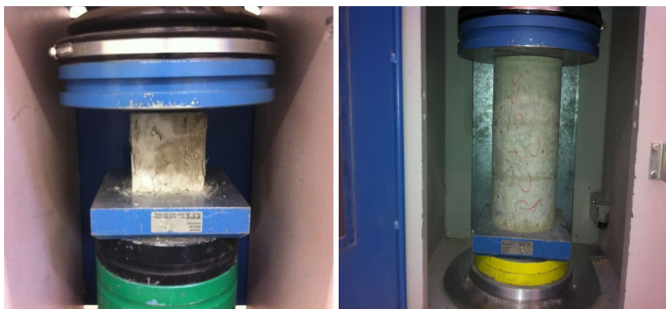
Figure 6. Compressive strength test using Avery Denison 2500 kN machines.
