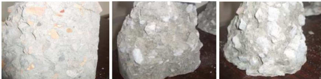
Figure 6. Failure plains of old mortars in RAC.
