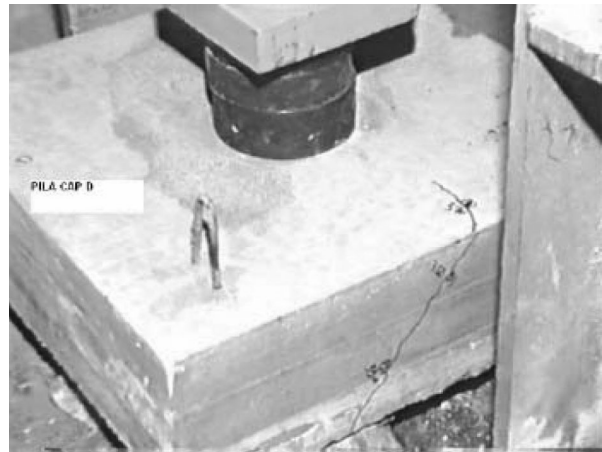
Fig. 5 Load applied at the centre of four-Pile cap. The Pile cap simply supported on four piles at the corner
