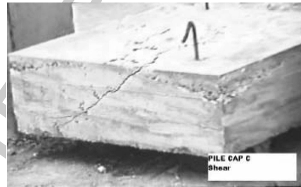
Fig. 5 Load applied at the centre of four-Pile cap. The Pile cap simply supported on four piles at the corner
