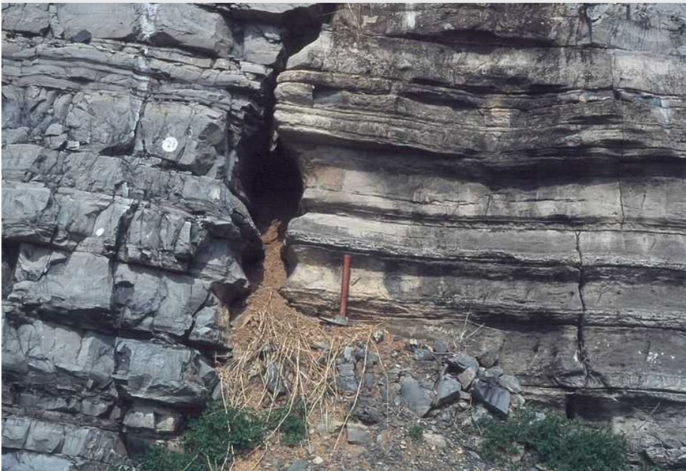
Comparison of un-weathered (left) and weathered (right) limestone.
