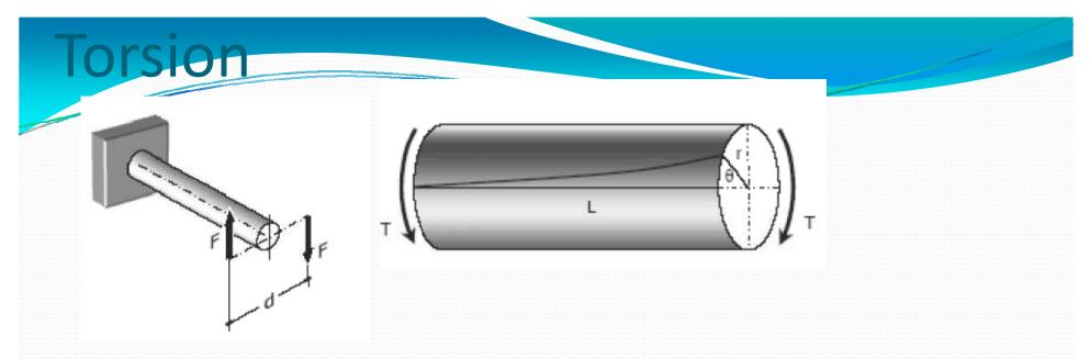
Torque or twisting moment T equivalent to  $F \times d$ , which is applied perpendicular to the axis of the bar, as shown in the figure. Such a bar is said to be in torsion.
