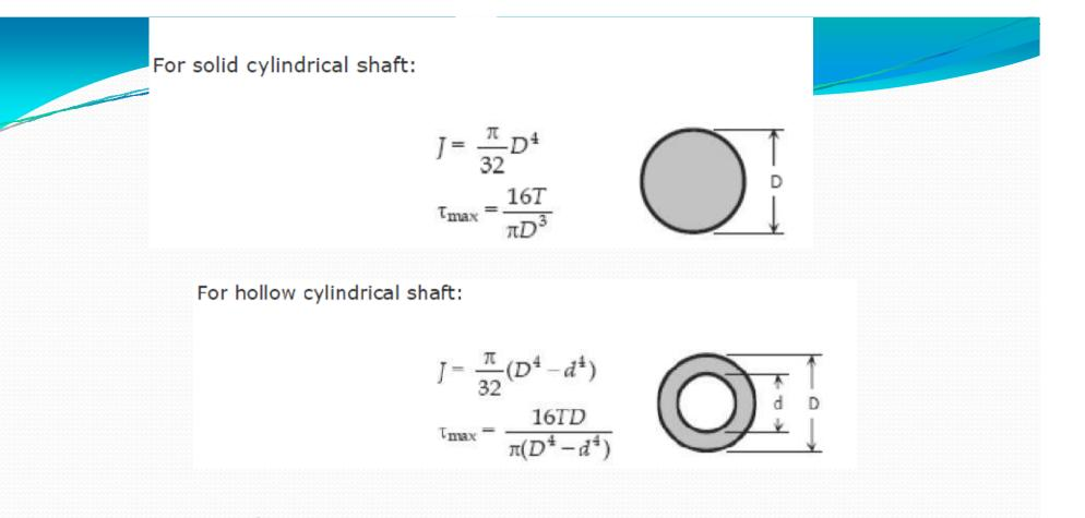
**ANGLE OF TWIST** The angle  $\theta$  through which the bar length L will twist is  $\theta = \frac{TL}{JG}$  in radians
