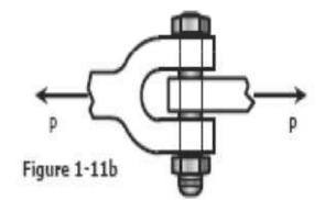
The bolt is subject to double shear.  $V = \tau A$   $400(1000) = 300[2(\frac{1}{4}\pi d^2)]$ d = 29.13 mm
